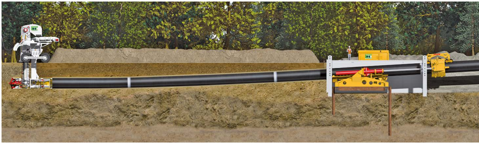
The push force delivered by Herrenknecht Pipe Thruster.
