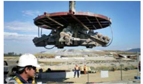
Reamer removal showing the use of a "false floor" providing safe working procedures.
