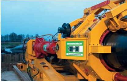
Pipeline embraced by the clamping device of the Pipe Thruster.
