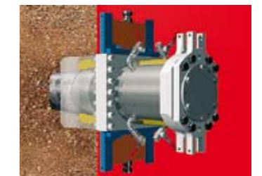
The cutter exchange is carried out from the rear via accessible cutting wheel arms.
