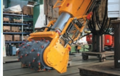
Cutting drum with special bits easily adaptable to different geological formations.
