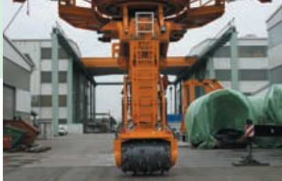
Telescopic boom with integrated cutting drum.
