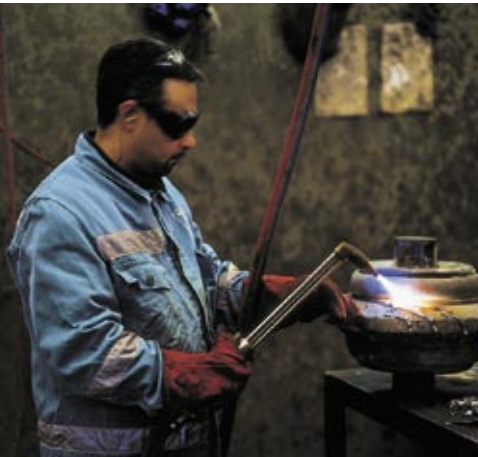
Dismantling of the Split Ring from the Hub.
