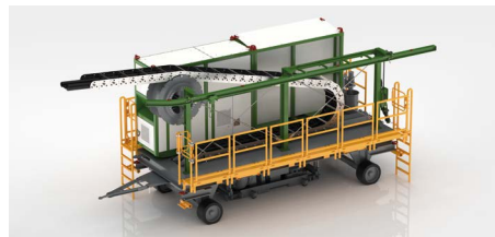
Support Unit accommodating peripheral equipment for drilling operation.
