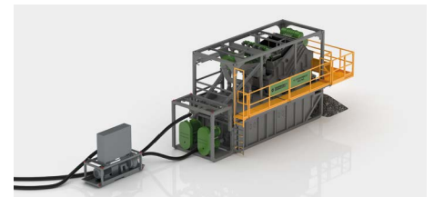
Slurry treatment plant and pumping system.
