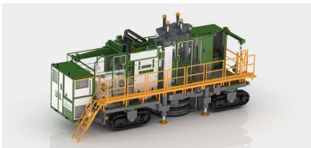
Self-propelled drilling rig accommodating drilling equipment.
