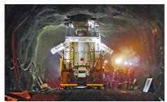
The modular design is adapted to limited drift dimensions.
