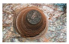
Successful launch: more than 60 holes have been produced so far with an average length of 16.5 m and an average advance rate of 1.5 m/h.
