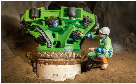
Reaming head on boring unit before collaring.
