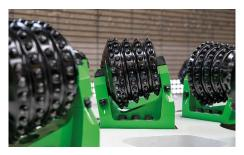
Raise Boring Cutter with tungsten carbide inserts.
