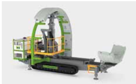
Fully mechanised installation of the lining elements.
