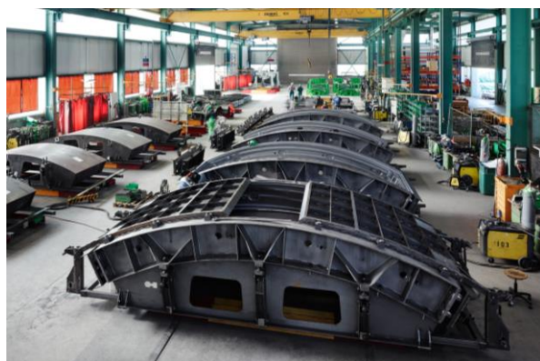
Photo 5: Herrenknecht Formwork supplied millimeter-exact moulds to the project for the production of concrete segments weighing 18 metric tons each.
