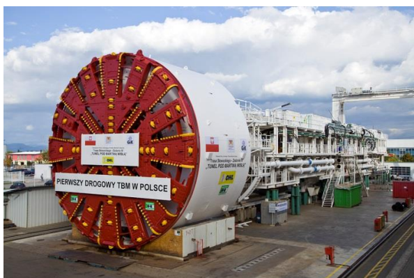
Photo 3: For the Slowacki tunnel project, Herrenknecht designed and delivered a 90 meter Mixshield with a shield diameter of 12.56 meters.
