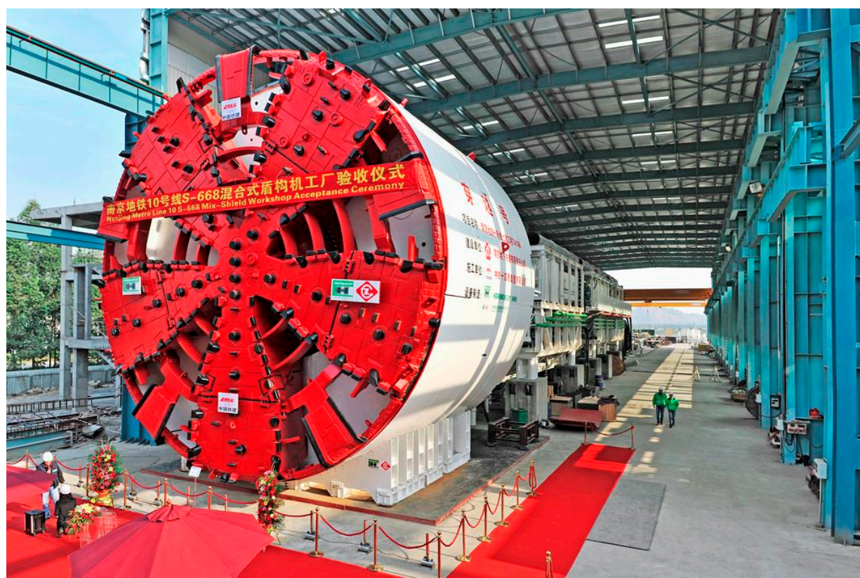
Picture 1: The Herrenknecht Mixshield S-668(Ø 11,610mm) on the occasion of its workshop acceptance in Nansha, Guangzhou, China.
