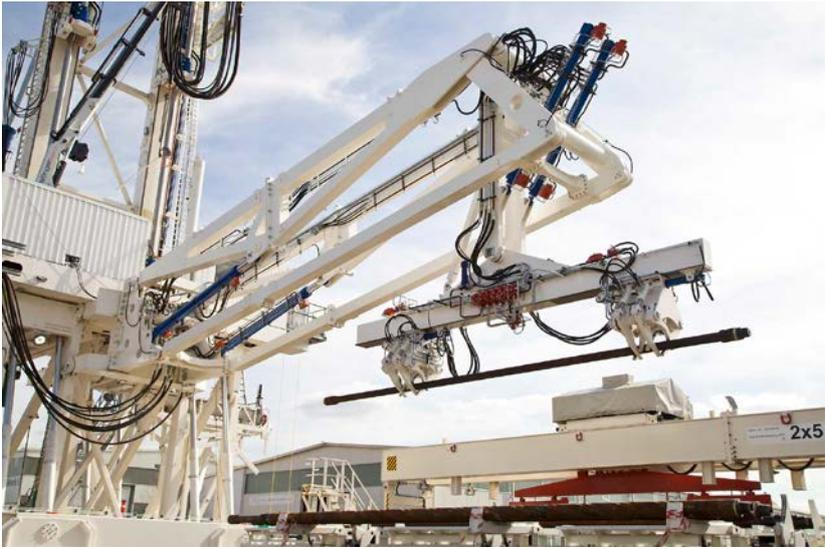
Image 2: The hydraulic pipe handler is used for hoisting the drill string and casing from the horizontal to the vertical drill axis. Hands-off technologies ensure a high degree of safety during the work process.
