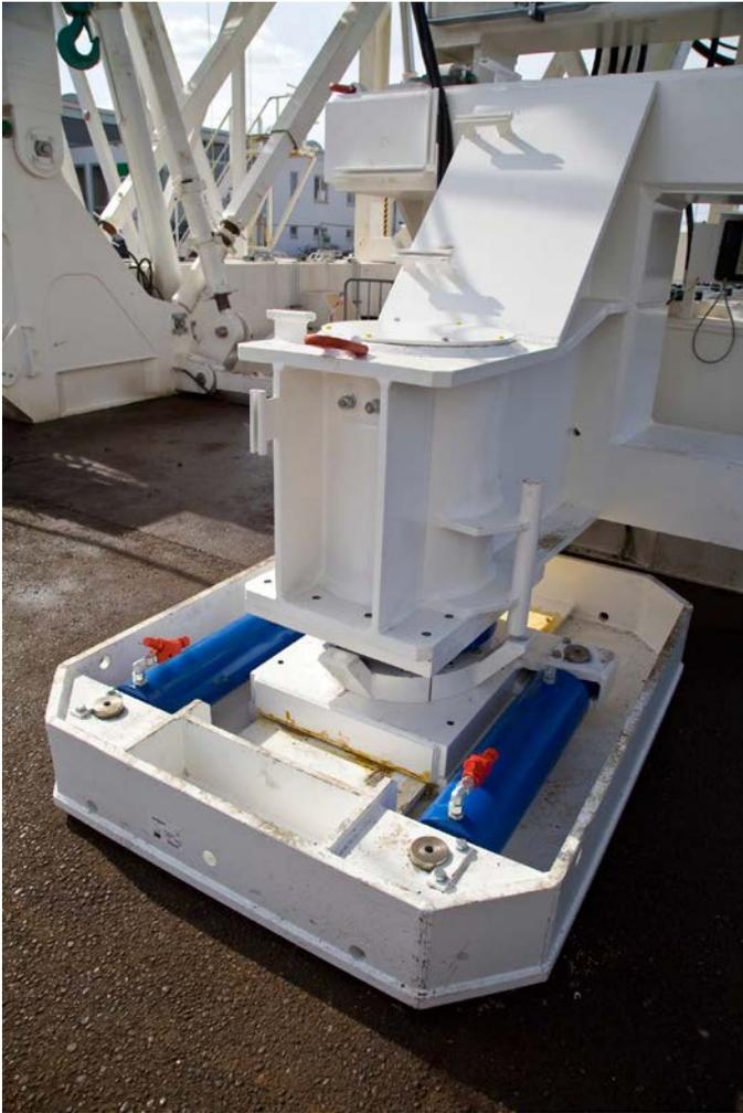
Image 1: Thanks to the newly-developed "X-Y Stepping" system with hydraulic cylinder supports, the deep drilling rig can be raised and skidded by several meters. This makes it possible to bundle several bore holes in so-called "multiple-well pads" as well as save time.
