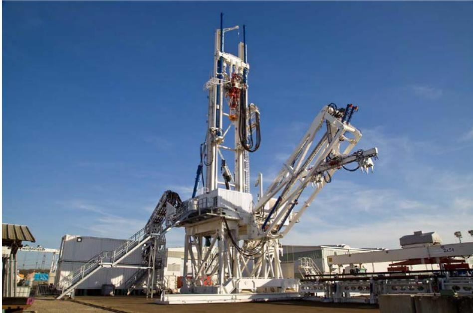
Image 3: All core pipe handling components such as the catwalk, pipe handler and hoisting system in the Terra Invader 350 plant are highly-automated and work very safely and precisely on the basis of the hydraulic drive concept.
