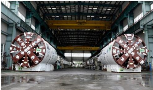
Called after districts in the city, the "Al Thummama" and "Al Rawada" machines with diameters of 4.47 meters and 121 meters in length, prior to delivery from the Herrenknecht plant. In Qatar, they are driving a 9.7 km tunnel under one of the main streets in the center of Doha's lively southwestern section while traffic continues to flow smoothly on the streets above.
