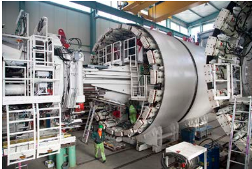
Photo 1: Plant assembly of the world's first Variable Density tunnel boring machines (TBMs) at Herrenknecht in Schwanau. They can be operated as an earth pressure balance shield and as a Mixshield. The variation of the density and hence the viscosity of the bentonite provides additional adaptability to tunnel face conditions.
