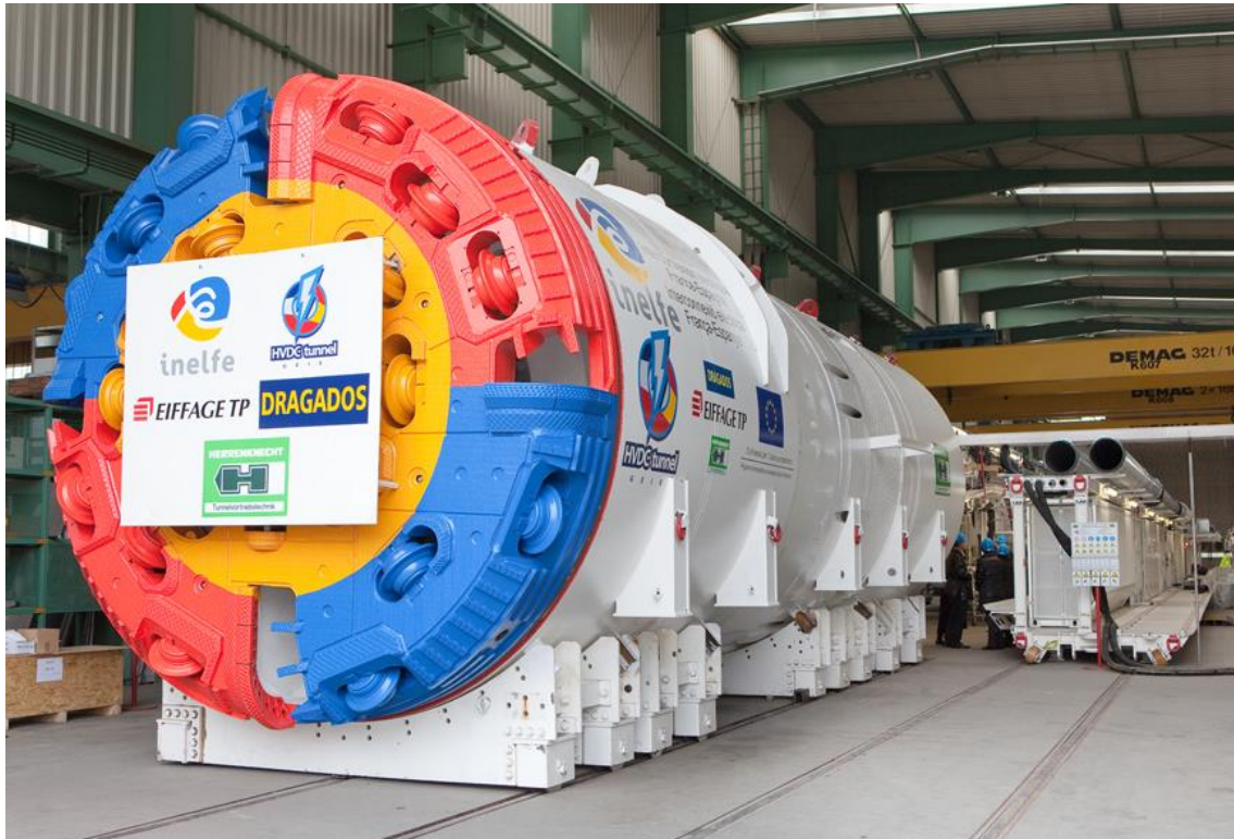
"Canigou" (M-1619M) - one of the two Herrenknecht Double Shield TBMs (Ø 4,256mm) for the excavation of the INELFE Tunnel project.
