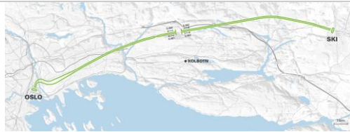
Photo 5: The two 20 kilometer long tunnels connect Oslo with Ski further to the south and from 2021 will shorten travel time for commuters by half.
