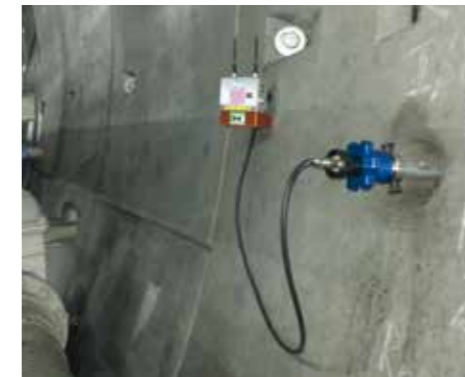
The WiFi data loggers at the end of the geophone anchors transmit the acquired data to the computer unit.
